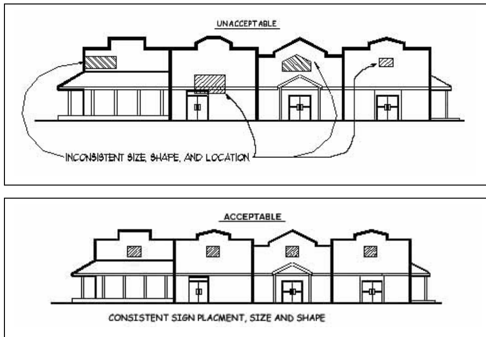
FIGURE 18B.180-2 – Wall Signage Placement
